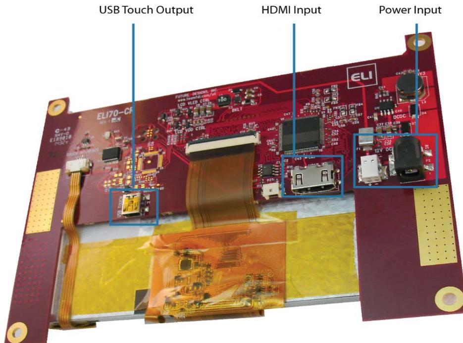
*Power may be supplied either via the 2-pin terminal block J8 or via the 2.1mm power jack P2 (center positive)*
