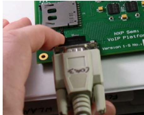
**Figure 2: Serial Connection**
