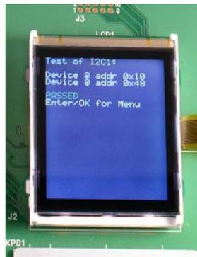
Figure 11: I2C1 Test
