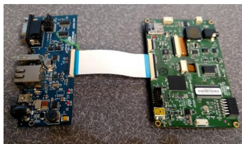
Figure 2: Attaching the Ribbon Cable
