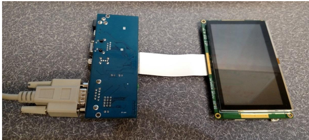
Figure 4: Connecting the RS-232 Cable
