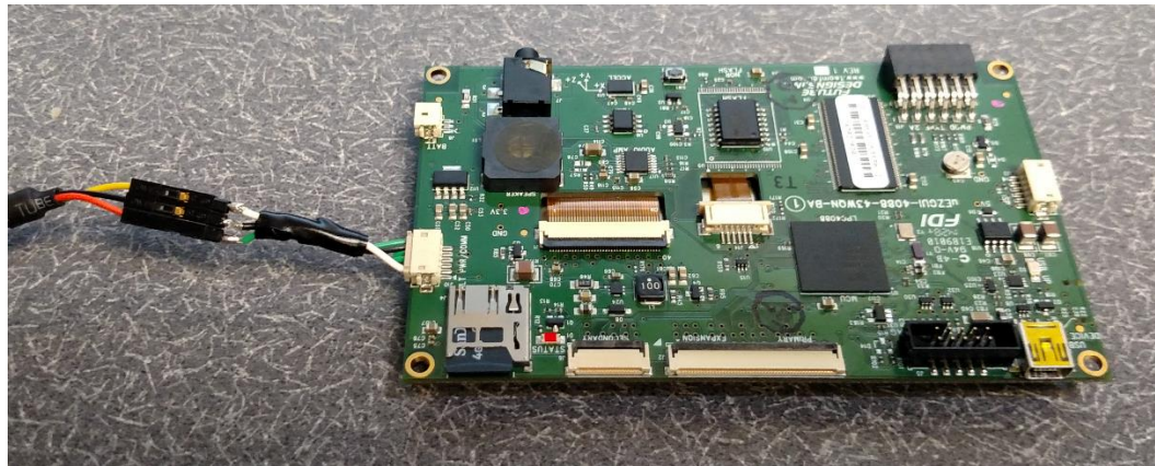
Figure 5: Connecting to the TTL UART
