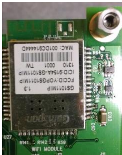
UEZGUI-1788-70WVM-BA Rev 1.1 with GainSpan Module (component view)
